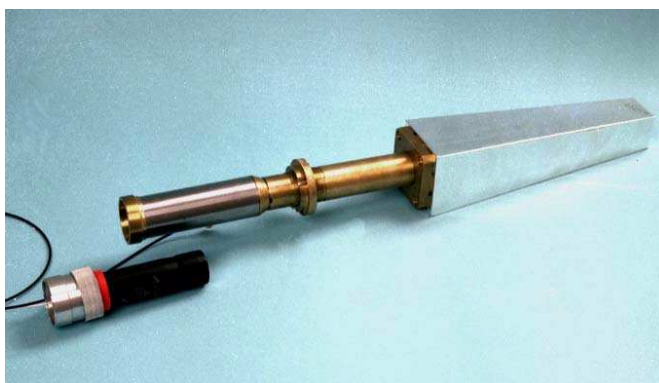
Figure 45: A fully equipped module with CsI crystal, light guide, PM tube and housing.
