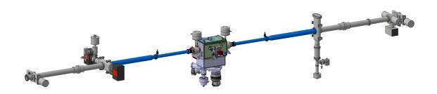
**Fig. 3.9.:** The complete PAX at COSY vacuum system. The NEG coated beam pipes, shown in blue, are connected to the target chamber. In addition the COSY section valve and ion getter pumps (red) are displayed.
