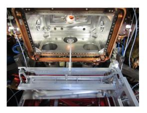
Fig. 3.15: Photograph of the open target chamber. Flow limiters have been installed at the entrance (left) and exit (right) of the chamber. The openable storage cell is shown in the foreground, affixed to a flange on which it slides into the chamber. The vertical tube on top of the storage cell is the feeding tube for the polarized atoms from the ABS. The long horizontal extension tube, connected to cell center, feeds the BRP on the backside of the target chamber.
