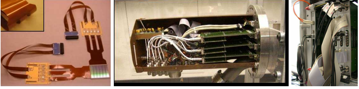
Figure 16: The developed electronic chain: In-vacuum boards with self-triggering chips (left panel), front-end interface boards (center), and complete vertex board with 12 bit ADC and sequencer (right panel).
