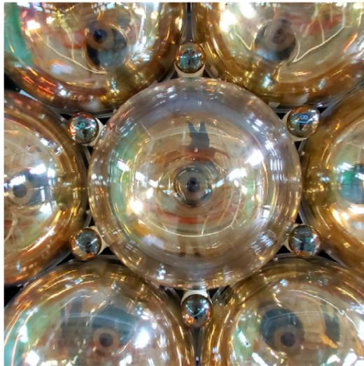
Figure 2.7: A real size mock-up of SPMTs interlaced with the LPMTs. From [39].
