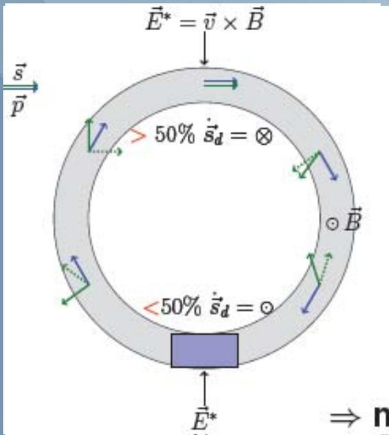
Solution; use of resonant „magic“ Wien-filter in ring ( $E+v \times B=0$ )
