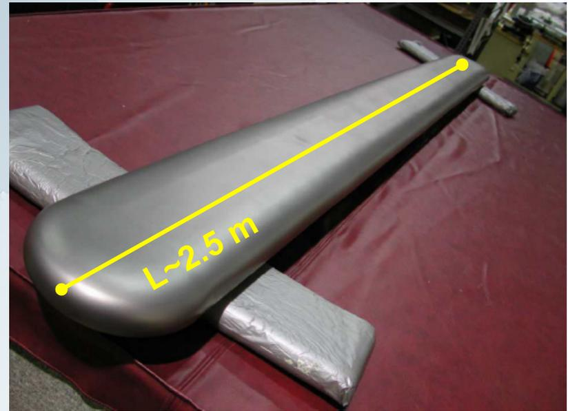
Routine operation at 1 spark/Year at 6 MV/m (180 kV at 3 cm)
