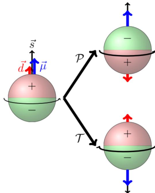
⇒ EDM measurement tests violation of fundamental symmetries  $\mathcal{P}$  and  $\mathcal{T}$  ( $\stackrel{\text{CPT}}{=} \mathcal{CP}$ )
