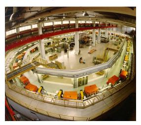
COSY provides (polarized ) protons and deuterons with  $p=0.3-3.7 \mbox{GeV}/c$
