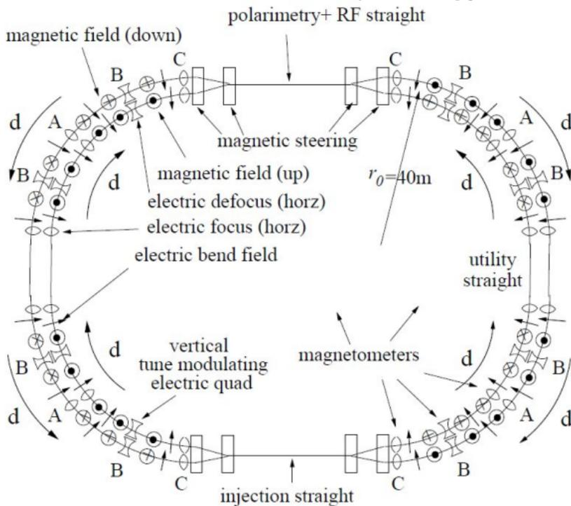
Figure 1: "All-In-One" lattice for measuring EDM's of protons, deuterons, and helions.
