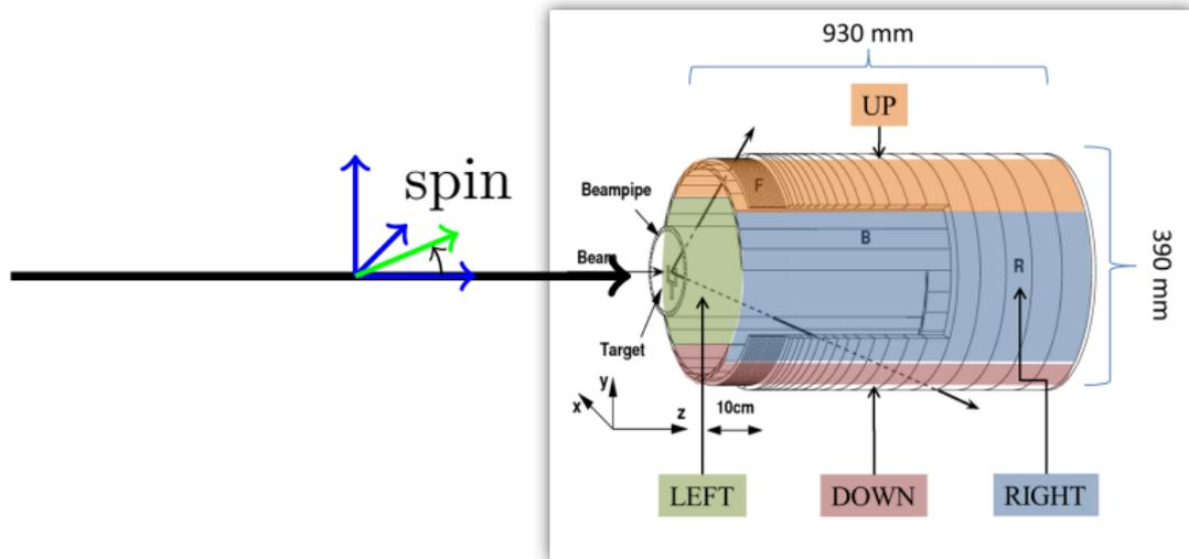
$$N_{up,dn} \propto 1 \pm PA \sin(\nu_s n_{turn}), \quad f_{rev} \approx 750 \text{ kHz}$$
