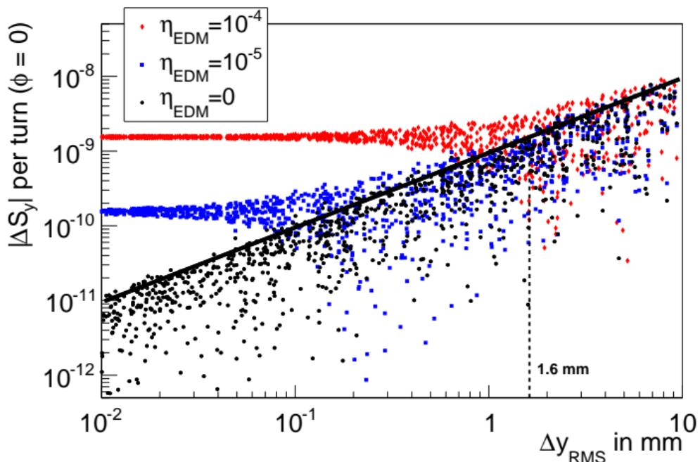
Random Misalignments from  $1 \mu\text{m}$  to  $1 \text{ mm}$
