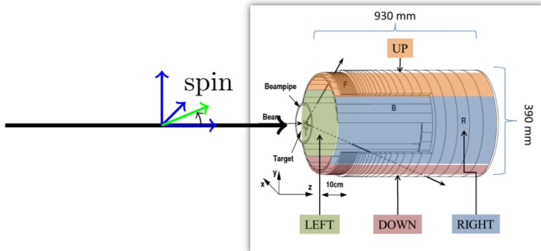
$$N_{up,dn} \propto 1 \pm PA \sin(\nu_s \omega_{rev} t), \quad f_{rev} \approx 750 \text{ kHz}$$
