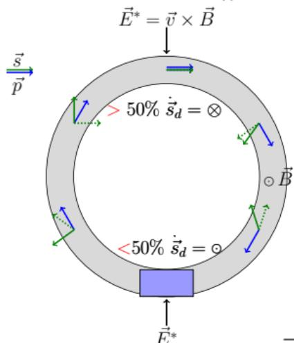
$E^*$  field in the particle rest frame tilts spin due to EDM up and down
