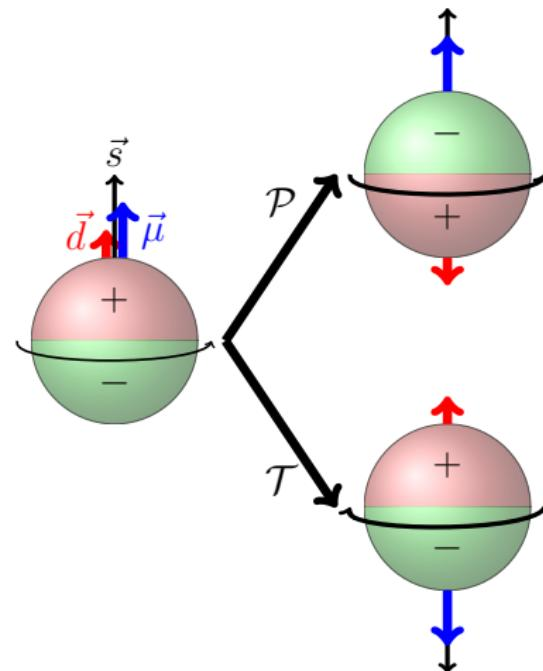
⇒ EDM measurement tests violation of fundamental symmetries  $\mathcal{P}$  and  $\mathcal{T}$  ( $\stackrel{\mathcal{CPT}}{=} \mathcal{CP}$ )
