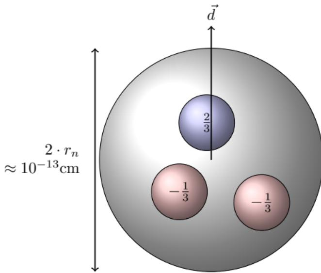
neutron EDM of  $d_n = 3 \cdot 10^{-26} \text{ e}\cdot\text{cm}$  corresponds to separation
