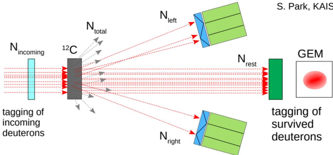
$$N_{\text{scattered}} = L \times \sigma_{\text{tot}} = N_{\text{el}} + N_{\text{inel}} = N_{\text{incoming}} - N_{\text{rest}}$$
