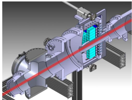
Cutaway drawing of the detector without the degrader (degrader is foreseen) and the plastic scintillator tracker.
