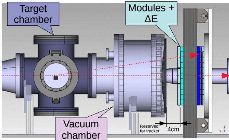
The JEDI polarimeter (JePo) inserted at the former ANKE detector location.
