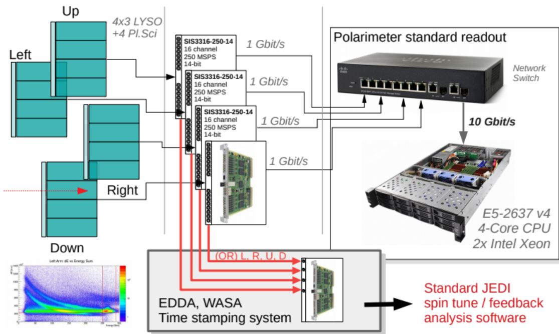
time stamping TDC readout are fed with OR signals from each polarimeter arm.
