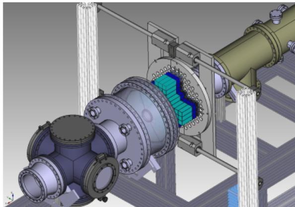
The JEDI polarimeter mounted on the support table. The crystals can be easily installed/repaired thanks to its openable support rods.
