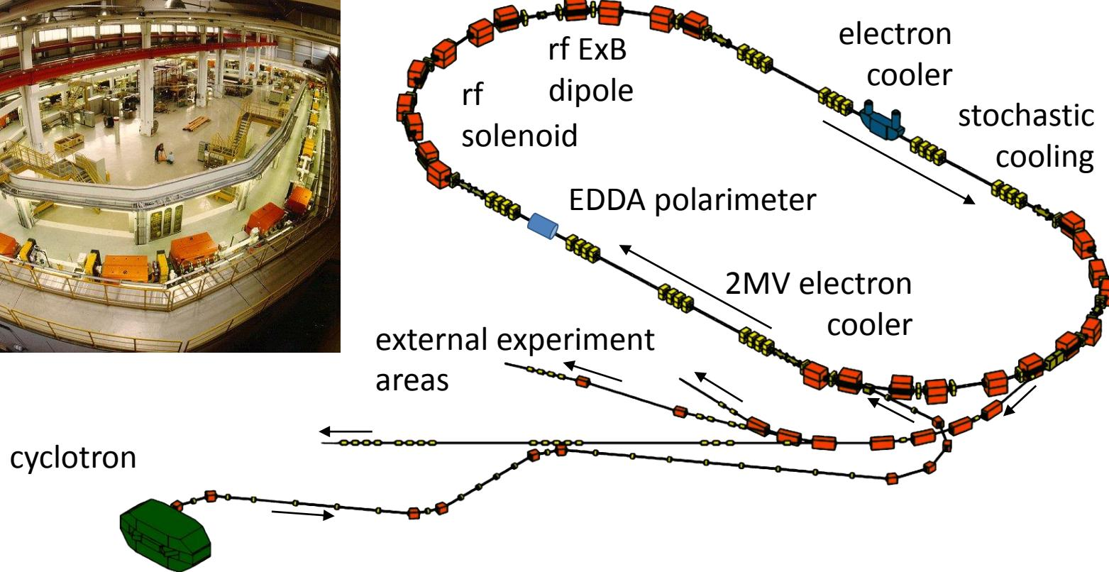
COSY provides cooled & polarized protons and deuterons with
