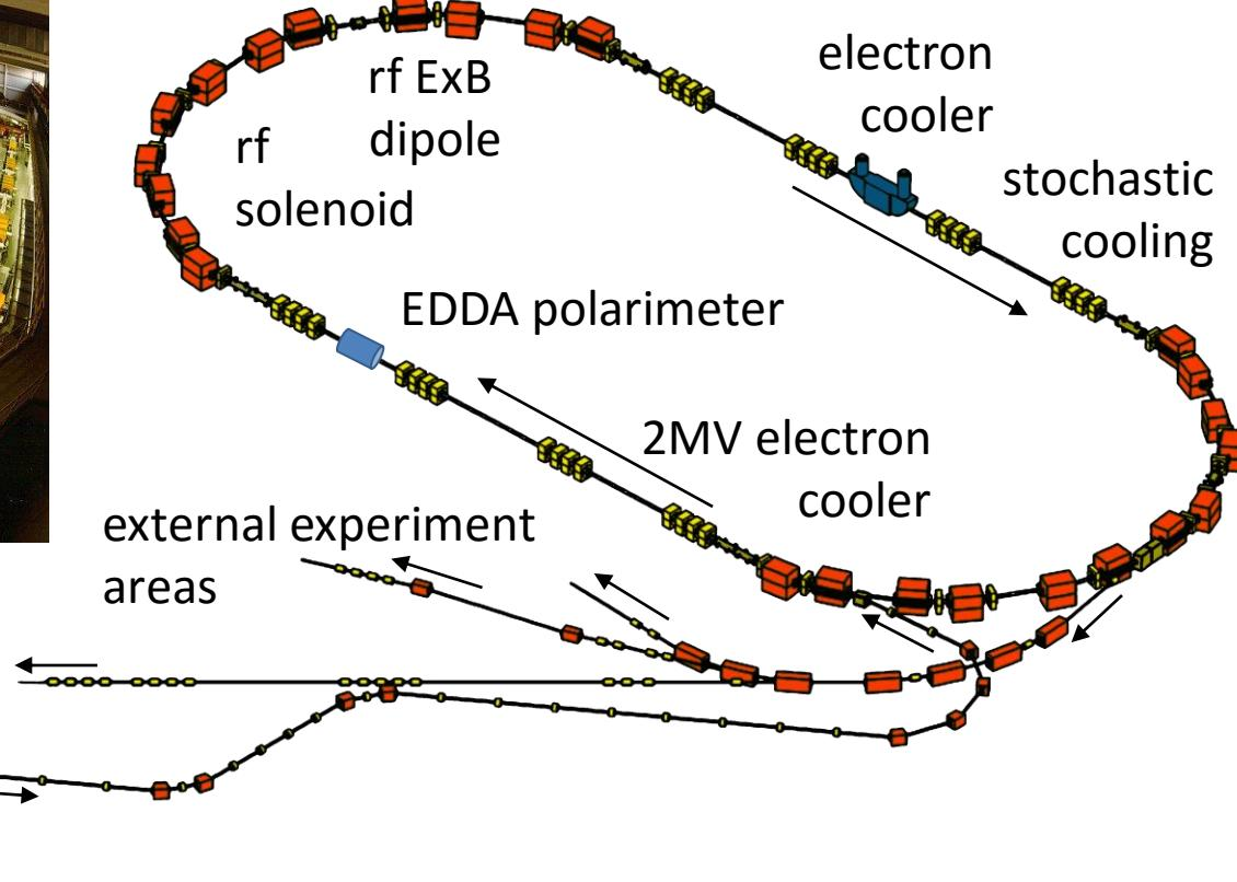
COSY provides cooled & polarized protons and deuterons with
