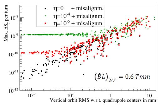
Uncorrected Gaussian distributed misalignments of the COSY lattice quadrupoles with a standard deviation of 0.1 mm generate a similar buildup as an EDM of  $d = 5.10^{-19}$  e cm
