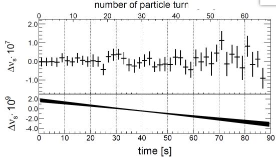
Spin tune  $v_s$  determined to  $\approx 10^{-7}$  in 2 s.  $\bar{v}_s$  in cycle at  $t \approx 40$  s is determined to  $\approx 10^{-10}$ . (submitted to PRL)
