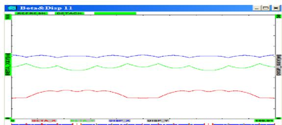
Figure 3: Twiss functions of electrostatic ring for ring and one cell
