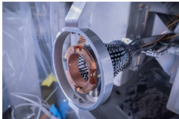
Openable storage cell at the SMOG internal gas target of the LHCb detector [16].
