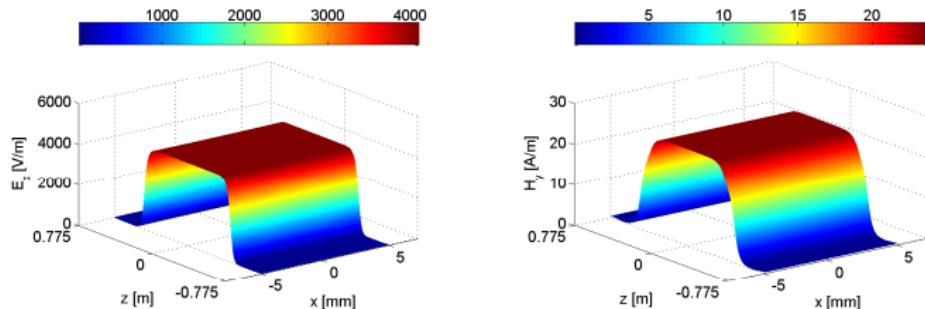
At input power of 1 kW, magnetic and electric field integrals ( $\ell = 1.550 \text{ m}$ ):
