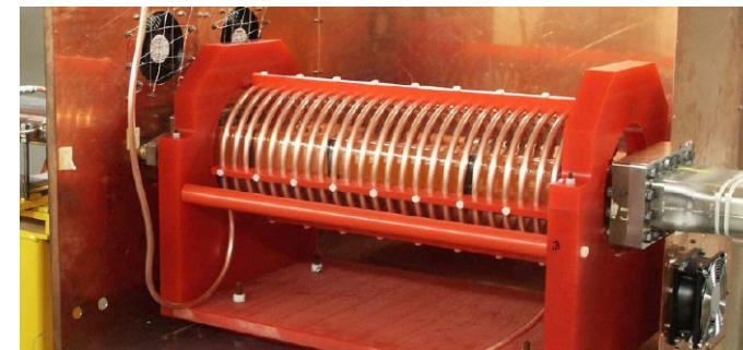
water-cooled copper-coil in ferrite box:
