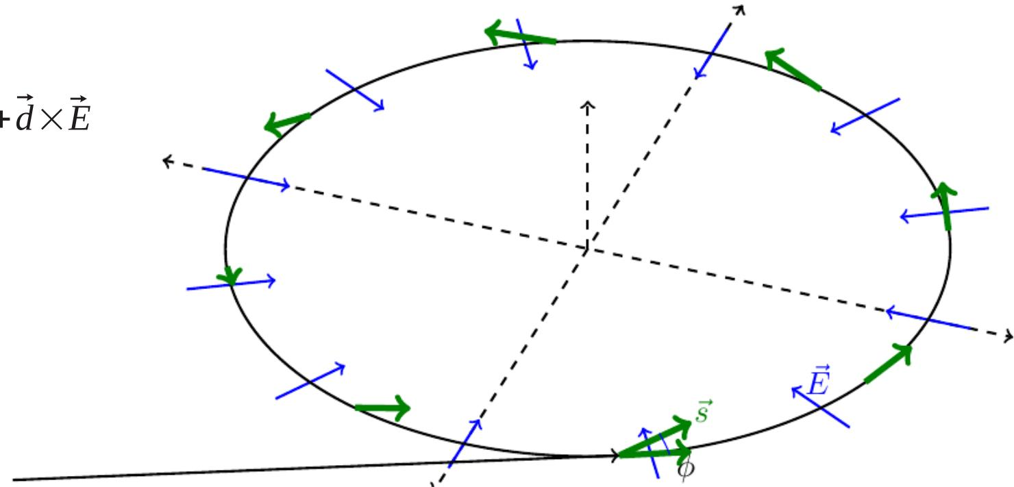
Initially longitudinal polarised particles interact with transversal electric field
