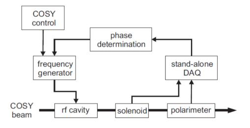
Use RF cavity to change spin tune via  $\nu_s=G\gamma$
