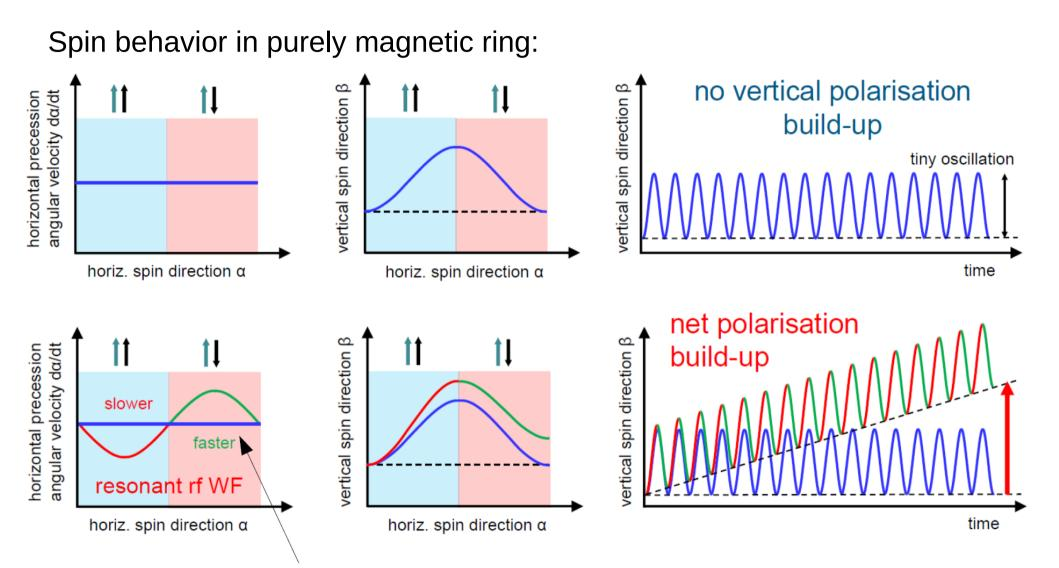
Wien Filter has to be always in phase with the horizontal spin precession! June 12th, 2018
