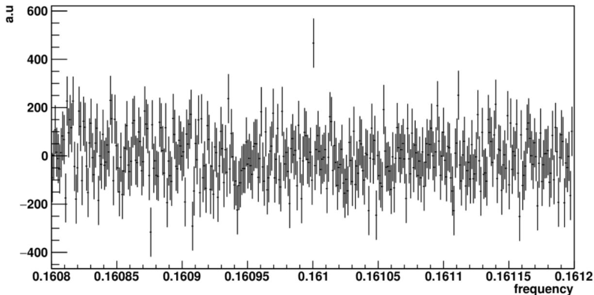
Analysing a much smaller frequency range, the Fourier spectrum shows clear peaks around the spin tune  $\nu_s = 0.16100045$
