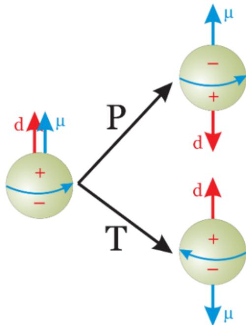
Figure: Behaviour of an EDM under P and T transformations
