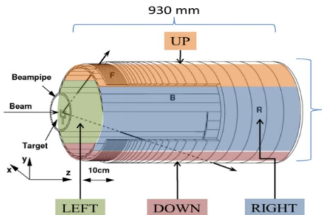
Figure: EDDA detector showing the separate detector quadrants
