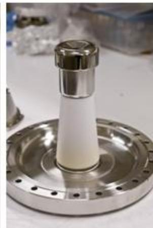
Replace conventional ceramic insulator with “Inverted” insulator: no SF<sub>6</sub> and no HV breakdown outside chamber
