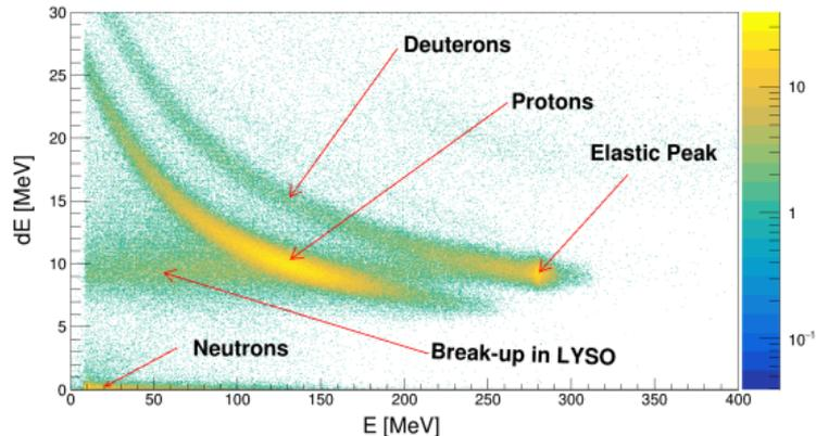
Resolution / dE vs E plot for PID
