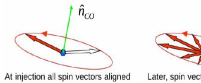
Later, spin vectors are out of phase in the horizontal plane
