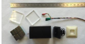
LYSO detector module, version I with PMT (left) and SiPM (right)
