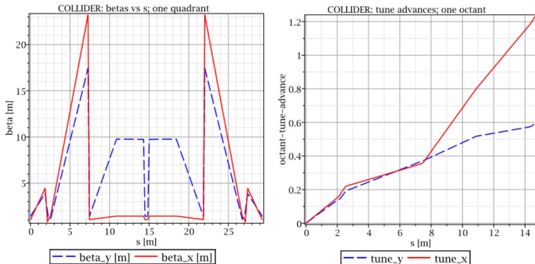
**Figure 6 :** Using “beta-squeeze” optics to reduce beta functions in both planes at the long straight section centers, countercirculating beams can be brought into a high luminosity collision configuration. This configuration can provide “beam-beam polarimetry” for EDM measurement consistency studies, or to measure  $pp$  and  $dd$  elastic scattering polarization dependence in the critical region below pion threshold, which is poorly understood at present.
