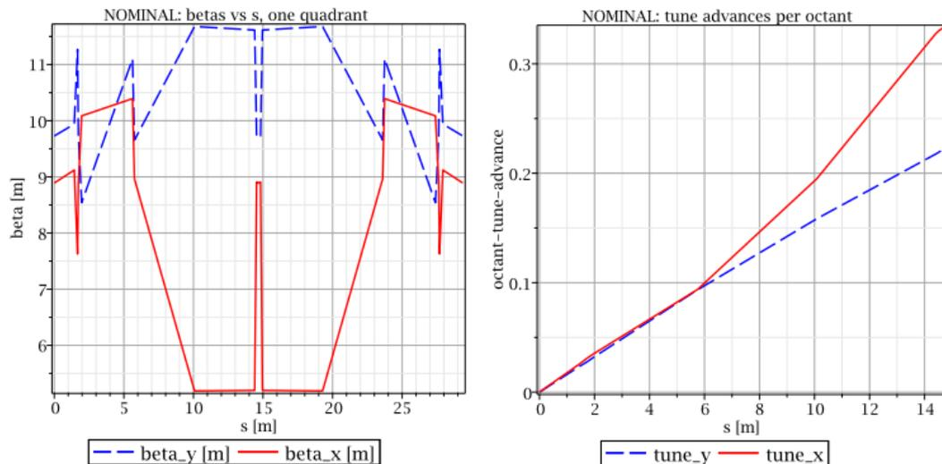
**Figure 4 :** **Left:** Same as previous figure, one quadrant PTR: NOMINAL beta functions, but plotted against longitudinal coordinate  $s$  assuming COSY beam hall installation. **Right:** Tune advances for one octant.
