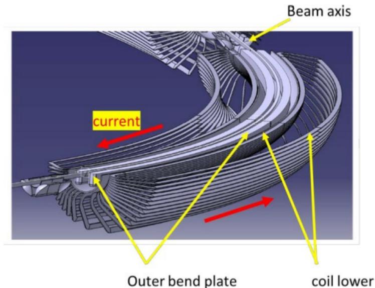
**Figure 1 :** Perspective mock-up of one quarter of PTR. Helmut Soltner design: partially-canceling nested coil,  $\cos \theta$ -dipoles coils. with “short-circuited” coil ends to cancel magnetic end-fields, surround the beam tube containing cylindrical electrodes.
