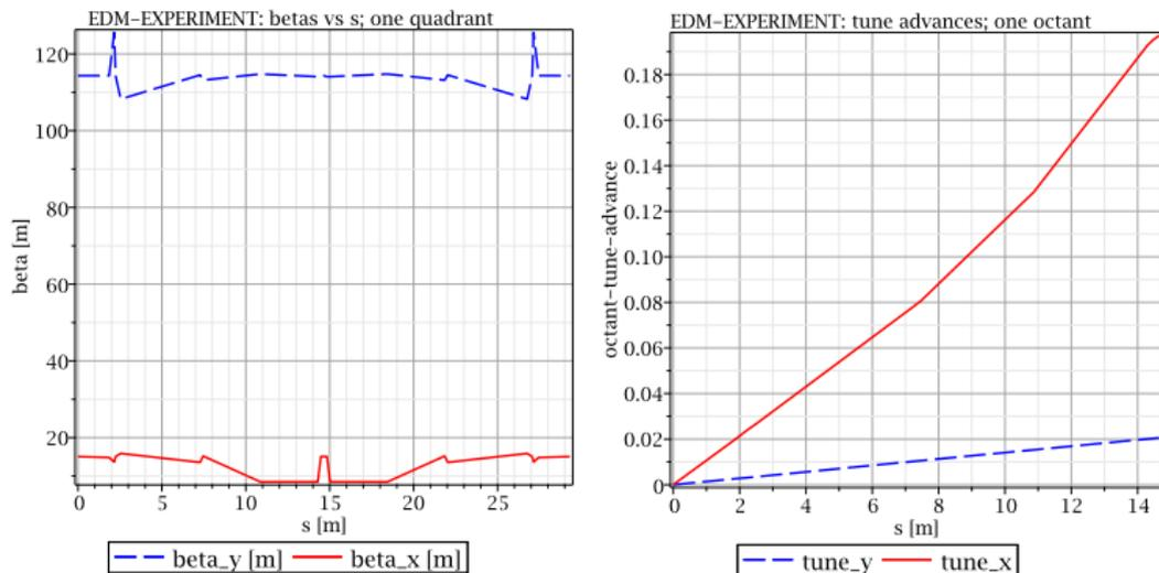
**Figure 5 :** Cancellation of  $\langle B_r \rangle$  depends on sensitive “self-magnetometry” (precision proportional to  $1/Q_y$ ) which requires small  $Q_y$ , and hence  $\beta_y(s)$  large for all  $s$ .
