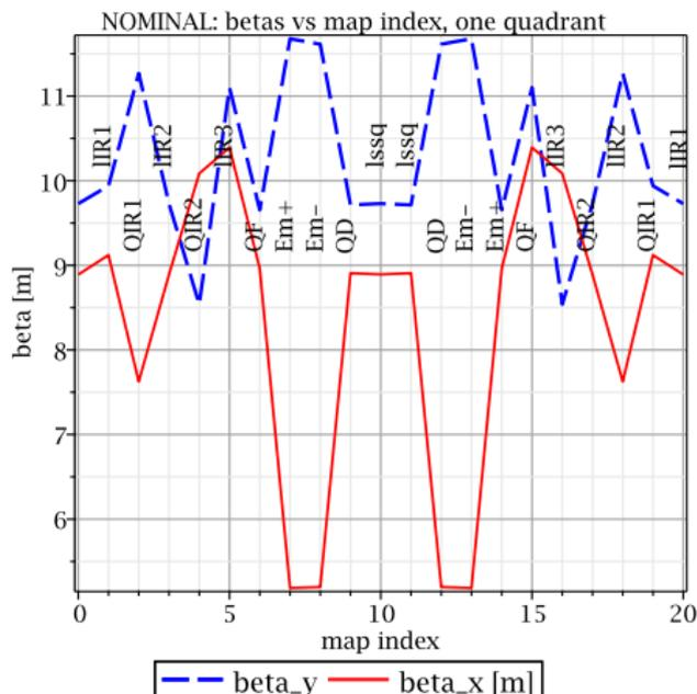
**Figure 2 :** Beta functions for one quadrant of the PTR-NOMINAL lattice. Note that the horizontal axis is element-index (not longitudinal coordinate  $s$ .) Element names are listed across the top. Solid (red) is horizontal, dashed line (blue) is vertical.
