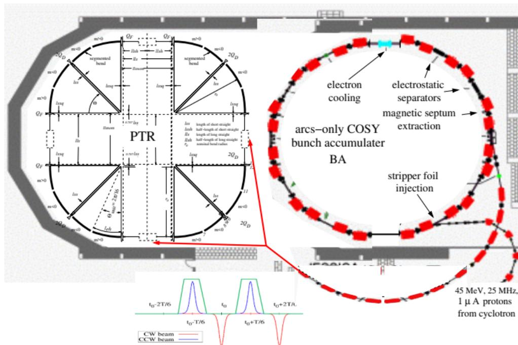
**Figure 3 :** If implemented in the COSY Hall, the bunch accumulator, BA, would be arcs-only COSY, rebuilt with existing electron cooling, stripper-foil injection and electrostatic-magnetic extraction.
