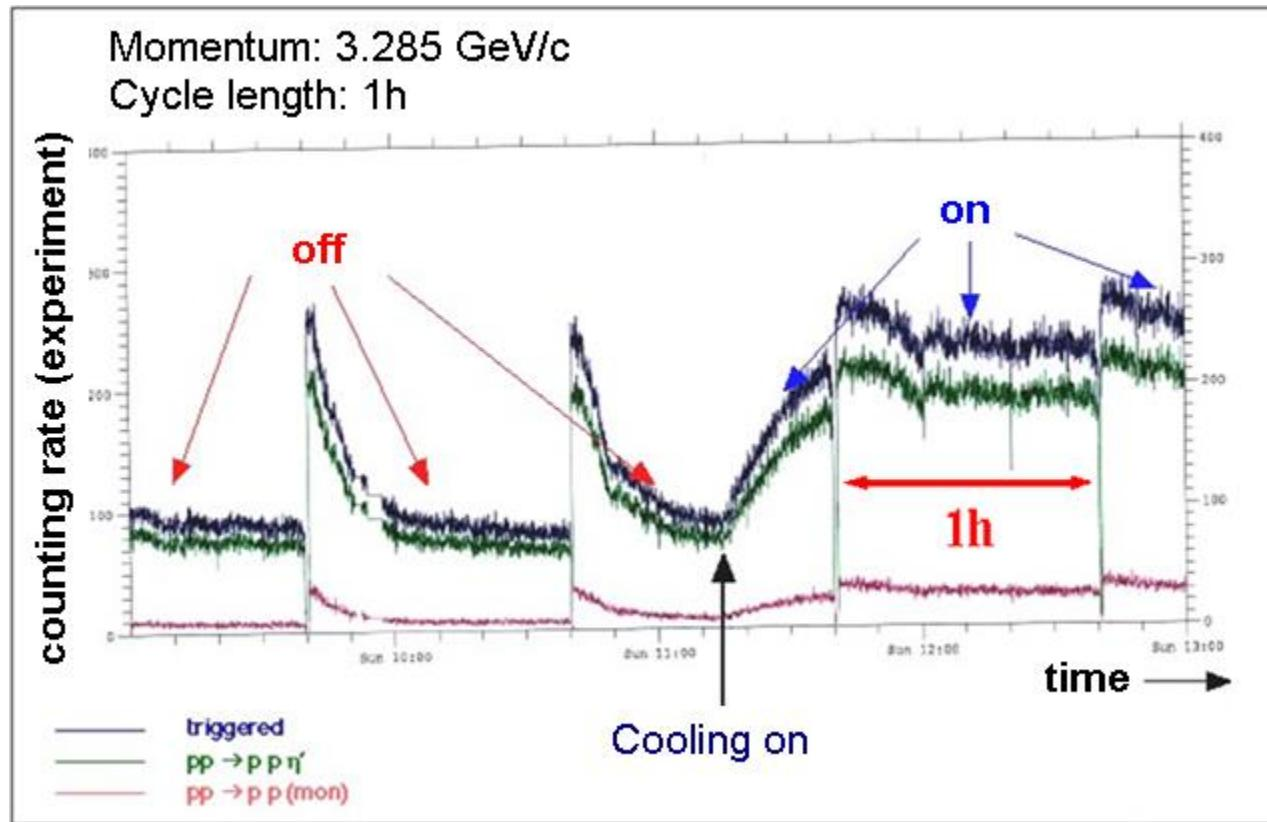
Compensation of emittance and momentum spread growth by an internal target
