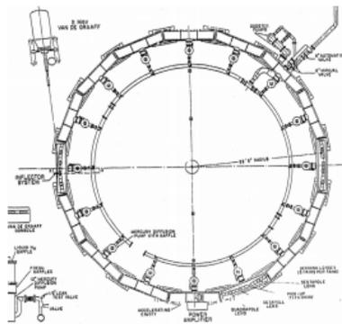
**Figure 1:** The 10 MeV “AGS-Analogue” electrostatic ring has been the only relativistic all-electric ring. It was built in 1954, for U.S.\$600,000. It could (almost) have been used to store 15 MeV frozen spin electrons. It was the first alternating gradient ring, the first to produce a “FODO neck-tie diagram”, and the first to demonstrate passage through transition (which was its *raison d’être*).
