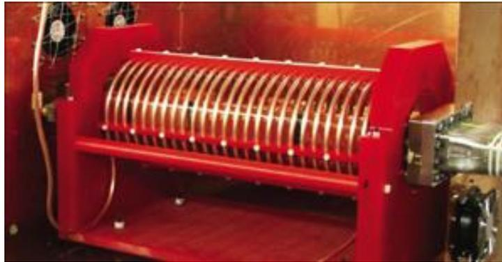
Figure 3.3: The RF Solenoid
