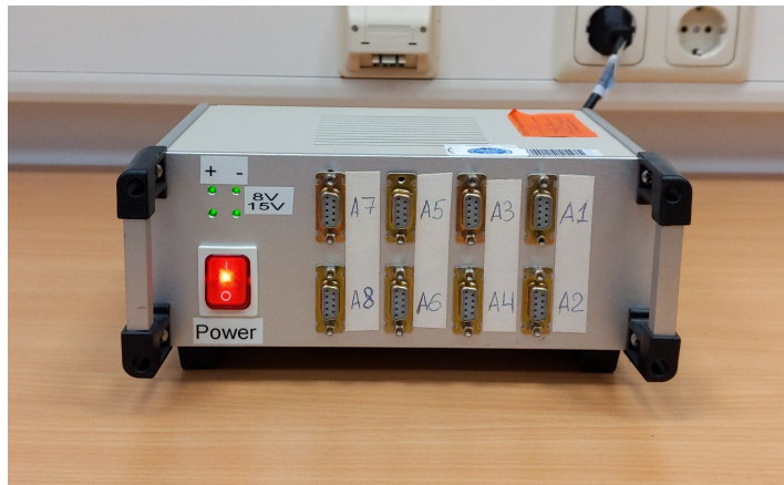
Figure 5.14: The power supply used to power the pre-amplifiers. The power supply is connected to a transformer to avoid the grounding to the mains.
