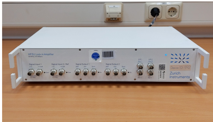
Figure 5.2: An image of the Zurich Instruments HF2 lock-in amplifier used in the BPM setup.
