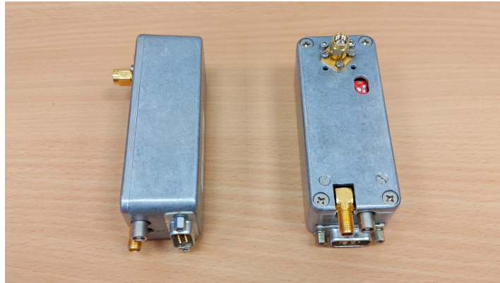
Figure 5.13: The pre-amplifiers used in the BPM setup. Switches visible on the underside of the pre-amplifier to the right.
