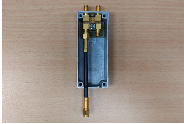
Figure 5.33: The box in this image takes one coil segment port (bottom) and splits it in to two port for the SVA input and output (top).
