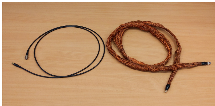
Figure 5.7: An image of the regular coaxial cable (left) and the shielded (with a braided copper sleeve) coaxial cable (right).
