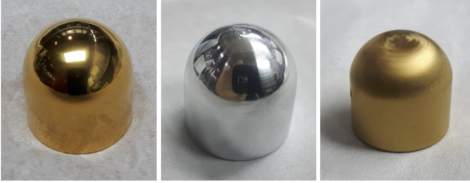
Figure 7: Three of the four different electrode types, all with a radius of 10 mm. From left to right: Coated stainless steel, aluminium and coated aluminium.
