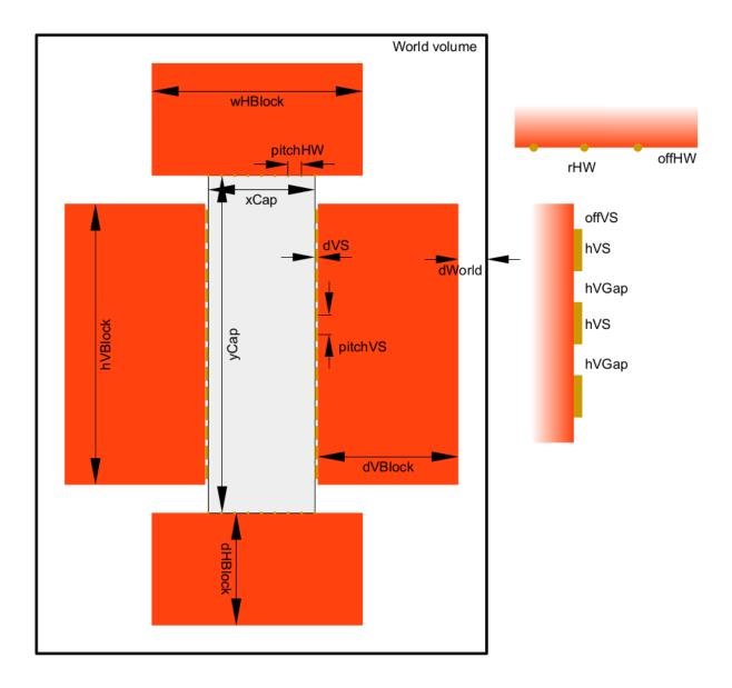
Figure 8: geometry in the deflector (see also in the annotations)
