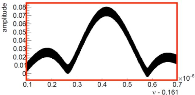
Amplitude of the Fourier transform in the 2nd turn bin in different frequency ranges. Note that both x-axes are offset by 0.161.
