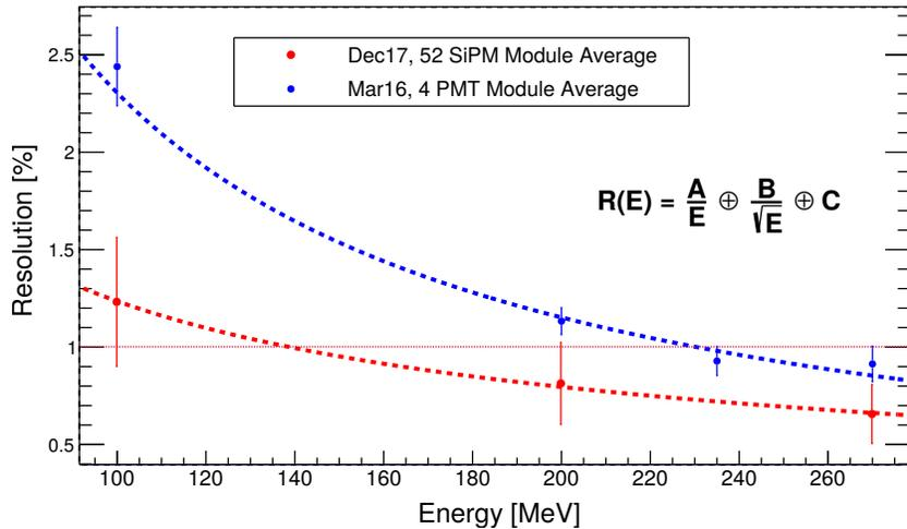
Figure 10: The comparison of energy resolutions as a function of incoming deuteron beam energy. Blue data points are a very first measurement of the LYSO crystals with PMT readout. The red data points are average of all modules with SiPM readout from December 2017 beam time. Note: here the resolution is defined as a FWHM over all modules divided by amplitude.
