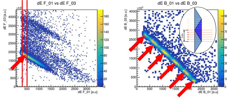
Figure 8: The amplitude correlation histograms for the forward and backward layers of two overlapping triangular scintillator bars. Left: a forward layer which is fixed relative to the beam and showing only the beam spread. The red lines show the cut area to choose a relatively focused beam for the second layer. Right: the correlation in the second layer while scanning along the overlapped side. The apparent correlation between the amplitudes is demonstrated.
