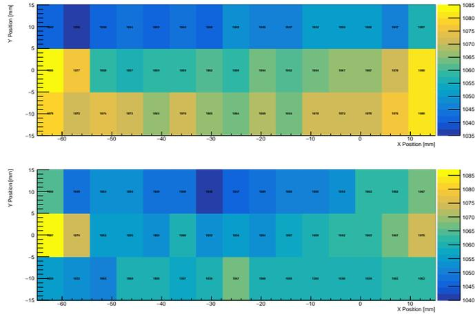
Figure 12: A  $15 \times 3$  side face map of a LYSO crystal at  $300MeV$  deuteron beam. In both measurements, the sensor is located on the right side. Upper: The same orientation as for the Fig. 11. Evident lowering of the light output can be identified in the upper part of the crystal. Lower: The  $90^\circ$  rotated map of the same crystal showing a different light output distribution from the upper face.
