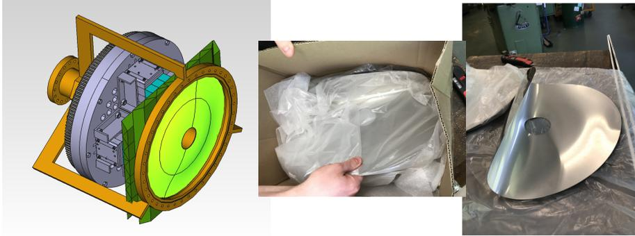
Figure 2: Damaged exit window during delivery.
