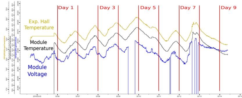
Figure 14: The module internal (black) and Big Karl experimental hall (yellow) temperature variation vs. time over the whole beam time. With the blue graph, the supply voltage for the same module is shown. The apparent correlation between all the values is evident.
