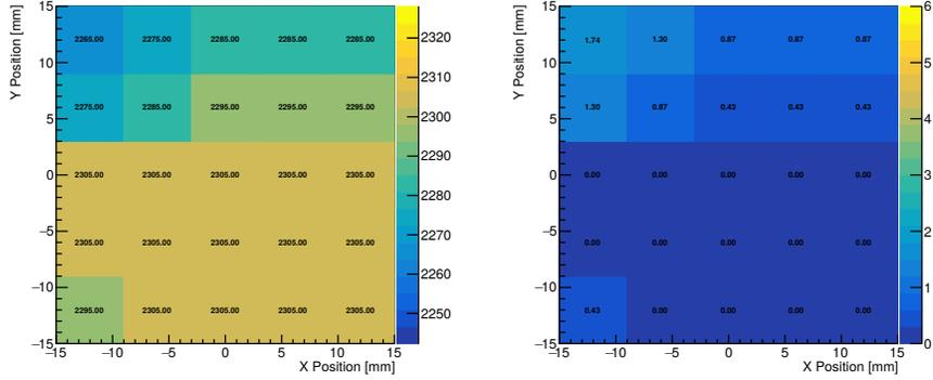
Figure 11: A  $5 \times 5$  front face map of a LYSO crystal with a  $300MeV$  deuteron beam. Left: the absolute values of peak position of the beam energy. Right: the relative deviation from the maximum value showing the homogeneity of the energy reconstruction to be within two percent.
