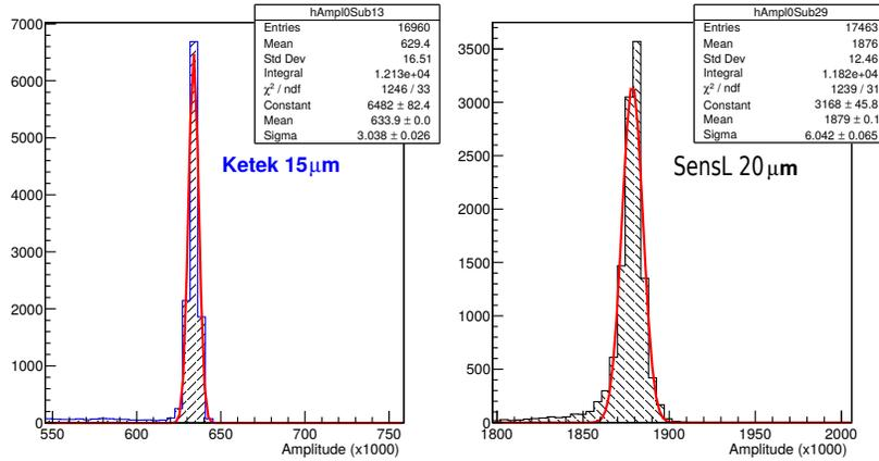
Figure 3: A typical charge distribution spectra at 200  $MeV$  deuteron beam energy aimed at the middle point of a crystal. Left: Ketek array with 15  $\mu m$  pixels at 29  $V$  and relatively low gain. Right: our standard SensL 20  $\mu m$  pixel array, also with 29  $V$  reverse bias voltage.
