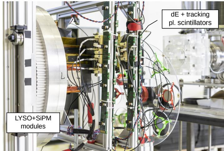
Figure 4: The experimental setup, similar to last beam time. In this setup, in addition to the last setup, six triangular plastic scintillator bars, three per plane, are used. The 2D scans of LYSO modules and the relative position scan for the plastic scintillators were made using this setup.
