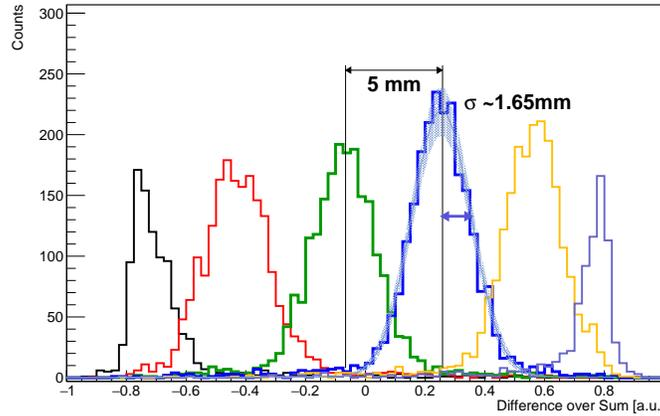
Figure 9: The difference over sum ( $\frac{A_1 - A_2}{A_1 + A_2}$ ) between the bars for six different positions along the overlapping sides (5 mm steps over a 3 cm side) of a backward layer is shown. Without much effort, the few millimeter resolutions can be achieved. This is a preliminary result from the online analysis. In the offline analysis we expect to reach millimeter level position resolution.
