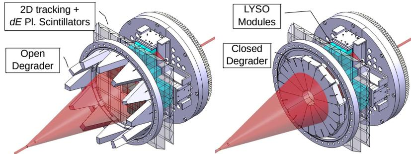
Figure 6: The JEDI polarimeter forward system consisting of the degrader system, the  $dE$  scintillating layer, and the LYSO modules. The  $dE$  layer consists of two layers ( $X, Y$ ) of overlaid triangular bars with  $2D$  position sensitivity.
