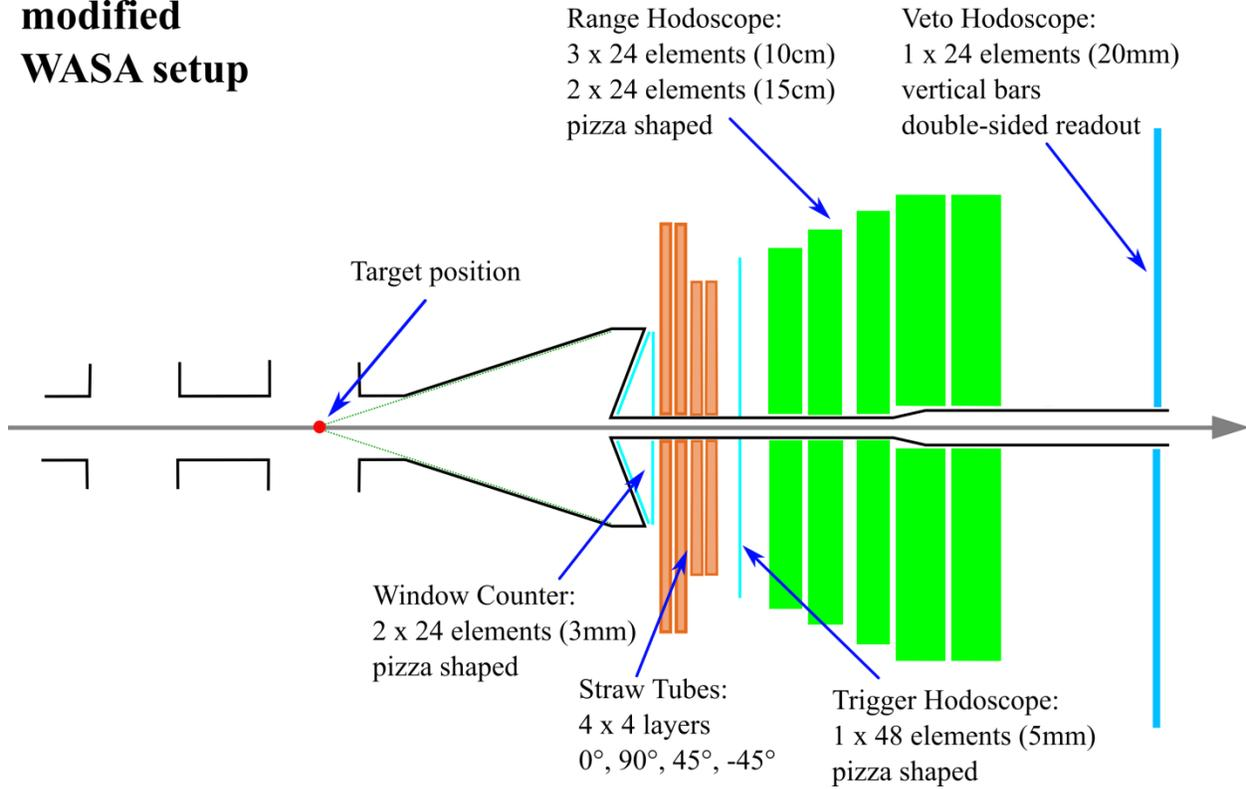
*Figure 1: A cross-sectional view of the Forward 17° detector from WASA as it may be configured in 2016 for the database experiment. The target position and various detector components are indicated.*
