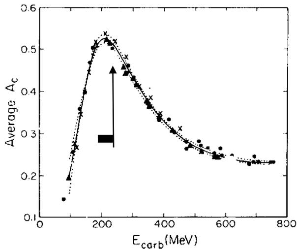
Figure 6: Values of the average analyzing power of a proton-carbon scattering polarimeter as a function of the proton energy. In general, passing scintillators were used in which the acceptance spanned the angles from the Coulomb-nuclear interference point (about  $5^\circ$ ) to an angle where the cross section is small enough not to matter ( $>16^\circ$ ). The arrow indicates the magic energy of 232.8 MeV. The box spans the energy of such protons in traveling through 5 cm of carbon.
