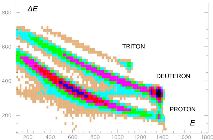
Figure 4: Particle identification spectrum of 110-MeV deuterons on a carbon target with a  $\Delta E$ - $E$  (plastic + NaI) detector telescope located at 27°. The bands represent tritons, deuterons, and protons going from top to bottom. Note the large flux of protons at roughly half of the beam energy. A reaction tail from the “energy” detector may be seen extending to the left of the elastic scattering peak at the end of the deuteron locus.
