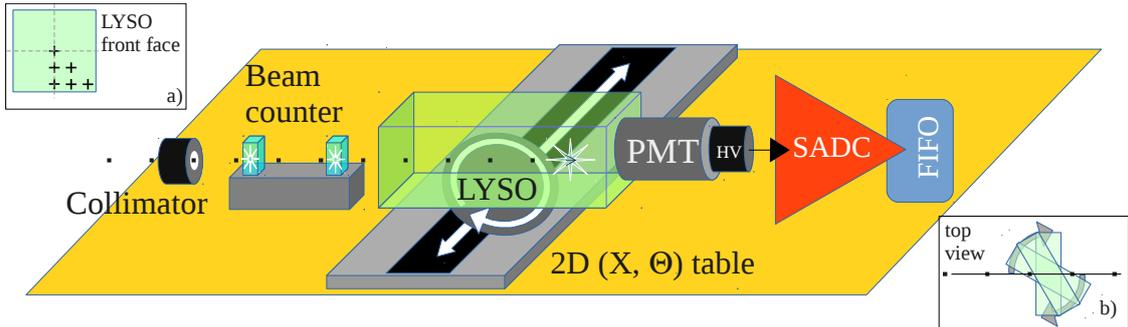
Figure 4: Test setup of the proposed first step measurement. Panel (a) shows the front face of the LYSO crystal and the six target points where the beam will be directed. Panel (b) demonstrates the rotation of the crystal in order to study the different energy losses by the deuteron to explore the Bragg peak distribution.
