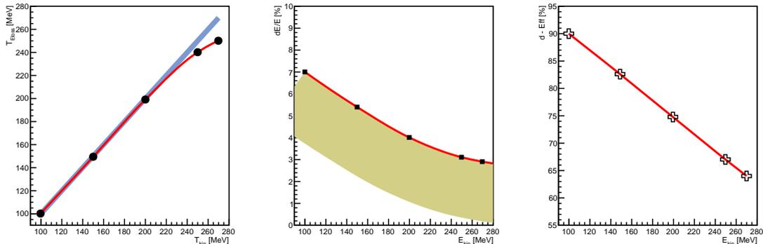
Figure 6: Simulated spectra: (Left) reconstructed energy; (Middle) measured energy resolution; (Right) elastic deuteron detection efficiency *vs* incoming deuteron beam energy (100, 150, 200, 250, 270 *MeV*).
