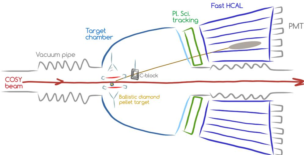
Figure 2: The sketch of the JEDI polarimeter.
