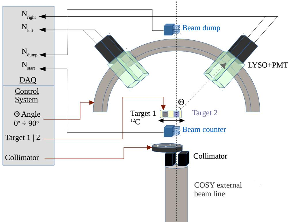
Figure 7: Supposed test setup of the second step measurement.
