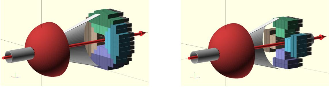
Figure 3: Left: The model of the final, full  $\phi$  and  $\Theta$  ( $5^\circ \div 20^\circ$ ) polarimeter; Right: its first simplified (with fewer elements) version and the outline of its vacuum chamber.
