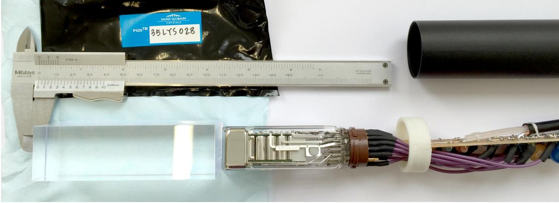
Figure 5: First sample of the LYSO crystal PreLude 420 produced by Saint Gobain [9]. The size of the crystal is  $30 \times 30 \times 100 \text{ mm}^3$ . The Photomultiplier tube (PMT) is a Hamamatsu R1548-07 [10].
