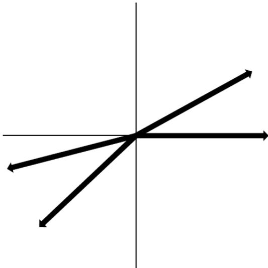
Figure 3: The relative polarization directions for the  $h=4$  bunches following precession from the vertical direction into the horizontal plane. By choosing the 870 kHz harmonic, every other bunch is nearly reversed in direction from the next bunch. Had this been done with the 630 kHz harmonic, all of the bunches would be grouped together into one quadrant of the diagram. The maximum opening angle (considering opposite directions as equivalent) is  $43^\circ$ .
