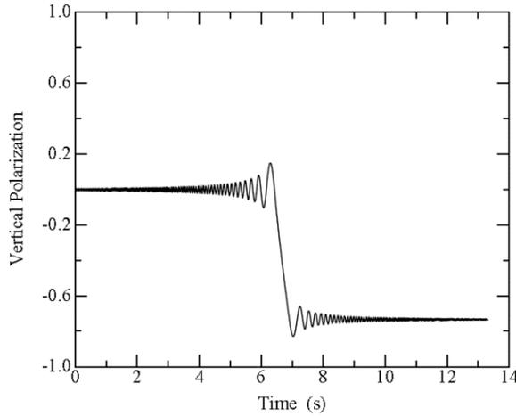
Figure 1: A “no-lattice” [14] calculation of the resonance crossing with a scan rate of 0.5 Hz/s. The strength of the oscillating EDM is  $1.6 \times 10^{-21}$  e·cm. Within the span of less than one second, this causes a jump of  $-0.75$  in the  $p[Y]$  component of the beam polarization (assumed to initially be completely polarized in the ring plane).
