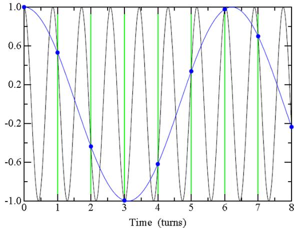
Figure 2: (left) A schematic diagram of the oscillations of the RF solenoid (black curve, 870 kHz) and an ideal beam polarization (blue curve) as a function of time in turns. Each turn is marked by a vertical green line. The blue dots indicate moments when the beam passes through the RF solenoid. (lower left) Same for beam passage through the solenoid halfway through a turn. (lower right) Same for  $\frac{1}{4}$  and  $\frac{3}{4}$  of a turn.
