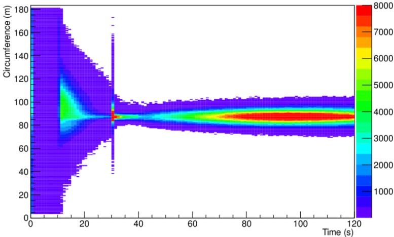
Figure 4: A graph of particle flux at the EDDA polarimeter as a function of time in the store and position around the ring circumference. Channels with less than 5 events/bin have been suppressed. The history shows injection, cooling, the start of DAQ, and a long storage time for gathering data. See the text for more details.
