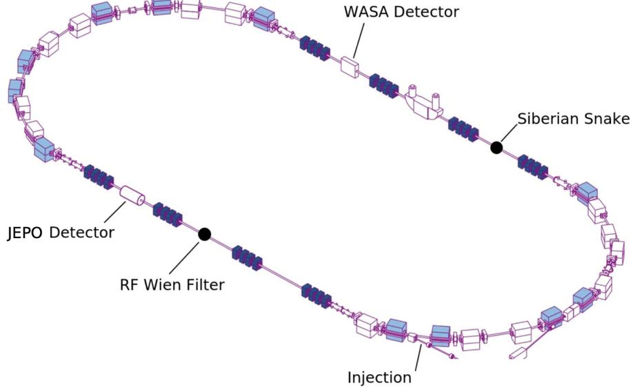
**Fig. 1.** The schematic of COSY showing the positions of the principal elements.
