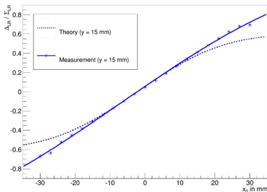
Figure 4: The ratio  $\frac{\Delta U_{LR}}{\Sigma U_{LR}}$  for the wire positioned at  $y_0 = 15$  mm and  $x_0 = -30$  mm to 30 mm. The dotted line represents the theoretical expectation, the solid line is a fit to the data points.
