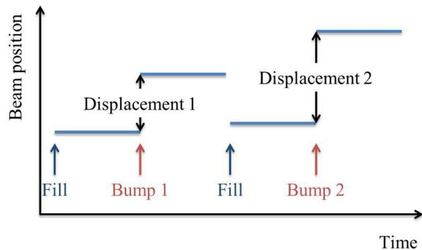
Figure 5: Schematics of the measurement sequence with two different local orbit bumps.
