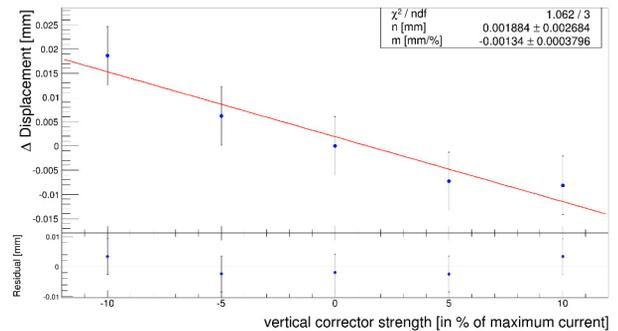
Figure 9: The measured horizontal beam displacement plotted against the corrector strength, which is proportional to the vertical beam movement.
