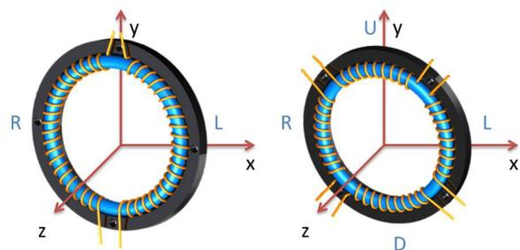
Figure 1: Half and quarter wound Rogowski coils in our coordinate system. The configuration shown on the left hand side permits a position measurement in  $x$ -direction. The configuration shown on the right hand side facilitates a measurement of the beam displacement in both directions:  $x$  and  $y$ .
