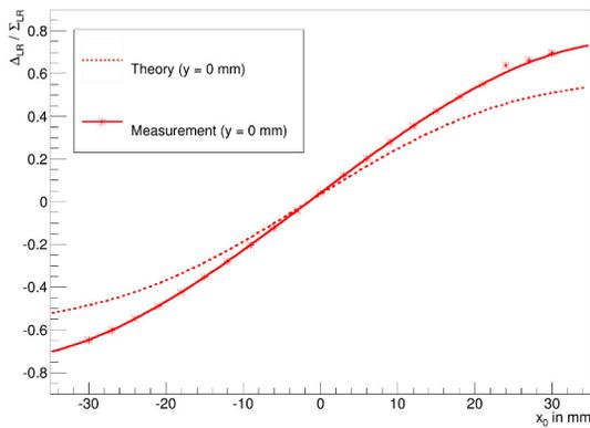
Figure 3: The ratio  $\frac{\Delta U_{LR}}{\Sigma U_{LR}}$  for the wire positioned at  $y_0 = 0$  mm and  $x_0 = -30$  mm to 30 mm. The dotted line represents the theoretical expectation, the solid line is a fit to the data points.
