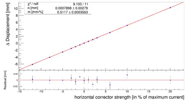
Figure 8: Test of the linearity of the BPM response to the corrector magnet excitation, which is proportional to a horizontal beam displacement at the BPM.
