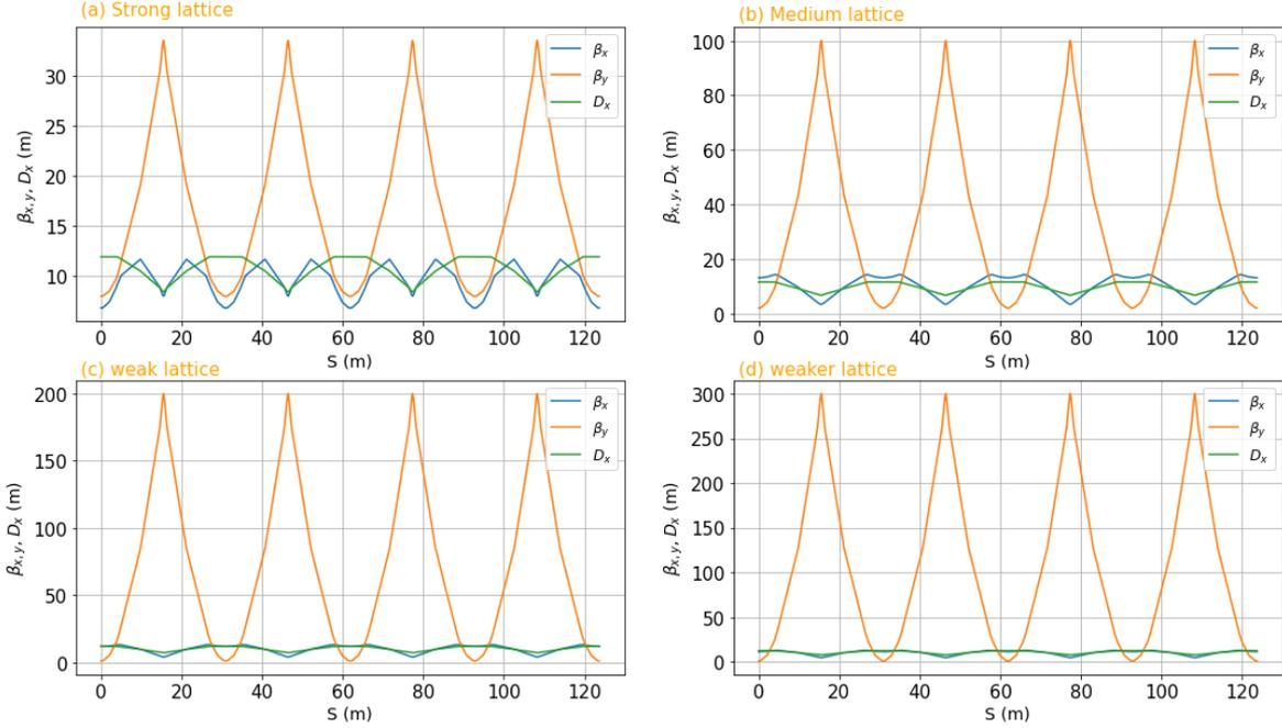
**Fig. 3.** Upper side : (a) is strong focusing lattice with  $\beta_{y-max} = 33$  m , (b) is medium focusing lattice with  $\beta_{y-max} = 100$  m , (c) is weak focusing lattice with  $\beta_{y-max} = 200$  m , (d) is weaker focusing lattice with  $\beta_{y-max} = 300$  m,  $\beta_x$  is horizontal beta function and  $D_x$  is horizontal dispersion
