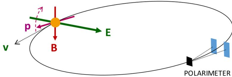
**Fig. 1.** Diagram shows a particle motion around the storage ring under the influence of electromagnetic fields. The polarization, initially along the particle's momentum, precesses towards the vertical direction in response to the radial electric field acting on the EDM. The vertical component of the polarization is observed through scattering in the polarimeter [2].
