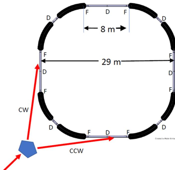
**Fig. 2.** Right side: The basic layout of the PTR, consisting of eight electrostatic deflectors, three families of quadrupoles (horizontally focusing: QF, horizontally defocusing :QD and straight section: QSS) and two families of sextupoles with total circumference of around 120 m
