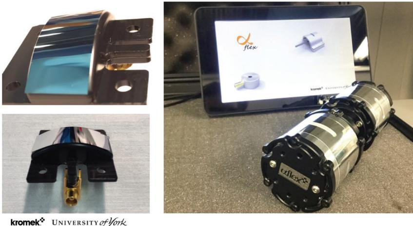
**Figure 1.** *Alphasflex pipeline inspection guide. The flexible silicon detectors are shown on the left hand side.*
