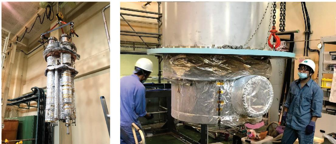
**Figure 4.** Preparation and installation of the He-II cryostat at KEK for testing. Left: cryostat internals. Right: nearing completion of assembly.
