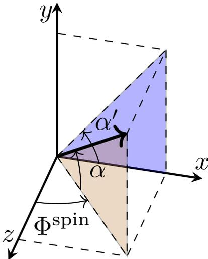
FIG. 1. Coordinate system used to describe the spin motion. The  $z$ -axis is defined by the nominal beam momentum, the  $y$ -axis points upward and the  $x$ -axis to the side.  $\alpha$  is the angle between the polarization vector and the horizontal plane.  $\alpha'$  is the angle between the projection of the polarization vector onto the  $xy$ -plane and the  $x$ -axis.  $\phi^{\text{spin}}$  is the phase of the spin rotation.
