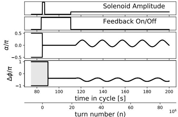
FIG. 2. Principle of the experiment.  $\Delta\phi$  can take any value in the shaded region.  $\alpha$  is initially  $\pm\pi/2$ . The first solenoid pulse tilts the polarization into the horizontal plane. The feedback system is then switched on to set a certain value of  $\Delta\phi$ . After that, the solenoid is switched on again at a lower amplitude and the feedback is switched off, leading to oscillations.
