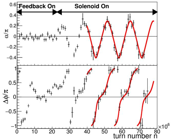
FIG. 6. Observation of unbound oscillation of  $\Delta\phi$ . The fit results correspond to  $k = (8.51 \pm 0.58) \cdot 10^{-7}$ ,  $q = 0.52 \pm 0.16$  and  $C = 0.205 \pm 0.087$  at a  $\chi^2/\text{NDF}$  of 82.8/74.
