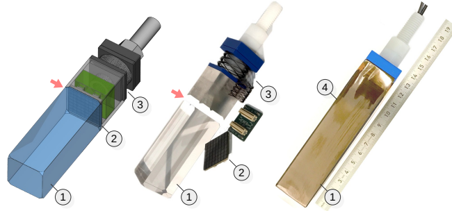
Figure 4. A full assembly sketch and disassembly photographs for a LYSO crystal detector with shading to indicate the main parts. The red arrows indicate where the corners of the LYSO crystal are chamfered to provide a stable mount against the aluminum housing that contains the SiPM. The labels indicate: (1) a LYSO crystal; (2) SiPM array ( 8 \times 8 ); (3) the housing and mechanical system; (4) wrapping with 3 layers: Teflon as a reflector, Tedlar to maintain light tightness, and Kapton [32] for mechanical stability.
