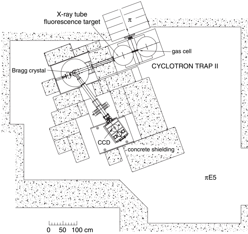
Fig. 3. Set-up for the pionic hydrogen experiment in the \pi E5 area at PSI. The concrete shielding of about 1 m thickness is essential to reduce the pion-induced background
