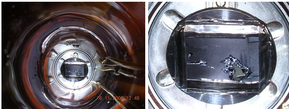
Figure 4.10: Left: View with the exit window removed into the cryogenic target cell. The solid GaAs target was mounted at the base. Right: Magnification of the GaAs target. The damage visible at the bottom right is discussed in Chapter 6.5.2.
