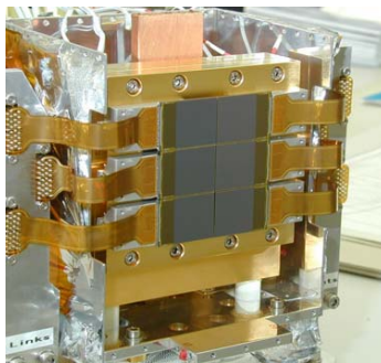
FIG. 1: Array of 6 CCD devices mounted on the cold head [7].
