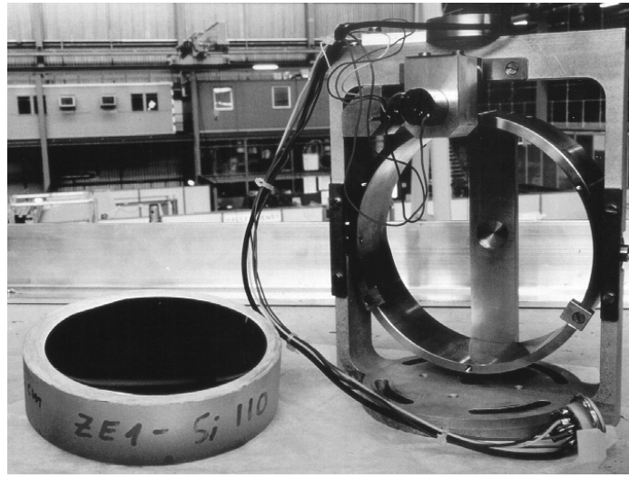
Figure 4.31: Photo of the crystal holder together with a Si(110) crystal at its side. The Si(111) crystal looks similar.
