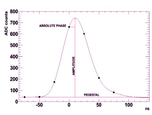
The analog signal from PMTs is shaped and sampled every 25 ns.
