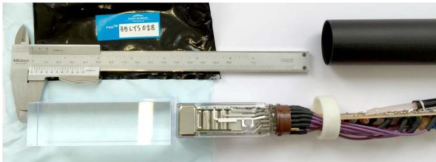
Figure 4: First sample of the LYSO crystal PreLude 420 produced by Saint Gobain. The size of the crystal is  $30 \times 30 \times 100$  mm<sup>3</sup>. The Photomultiplier tube (PMT) is a Hamamatsu R1548-07.
