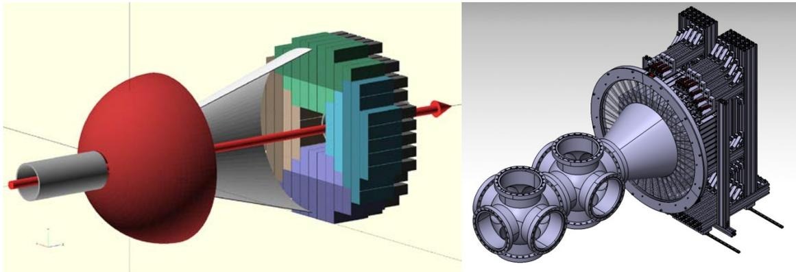
Figure 2: The GEANT simulation model of the final polarimeter (left panel) and its current engineering model (right panel).
