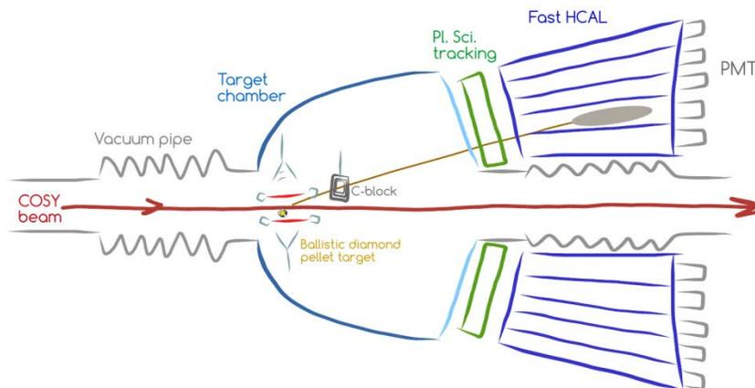
Figure 1: The sketch of the JEDI polarimeter.
