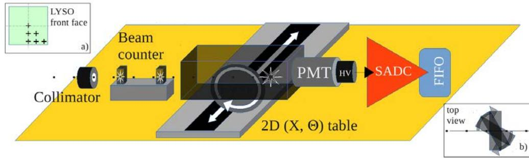
Figure 3: The test setup of the first step measurement. Panel (a) shows the front face of the LYSO crystal and the six target points where the beam will be directed. Panel (b) demonstrates the rotation of the crystal in order to study the different energy losses by the deuteron to explore the Bragg peak distribution.
