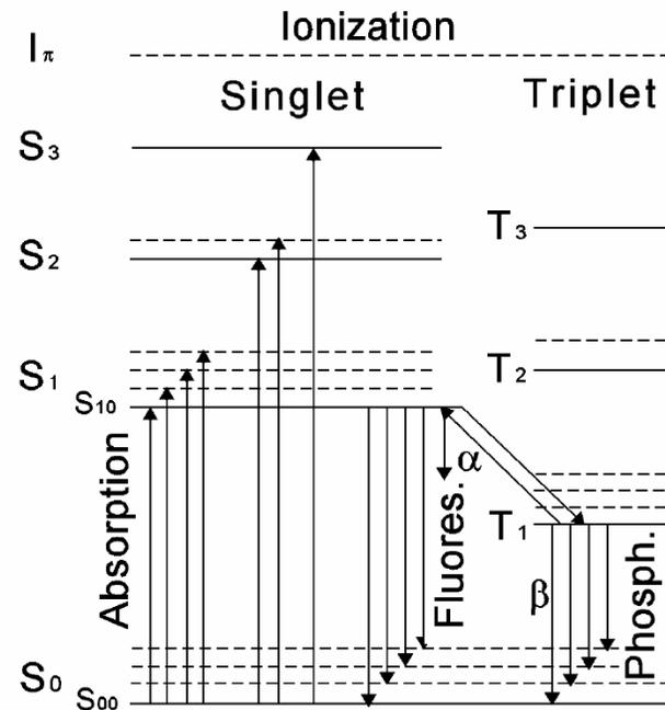
Emission of scintillation light. Its amount is  $f(\text{deposited energy, particle type})$
