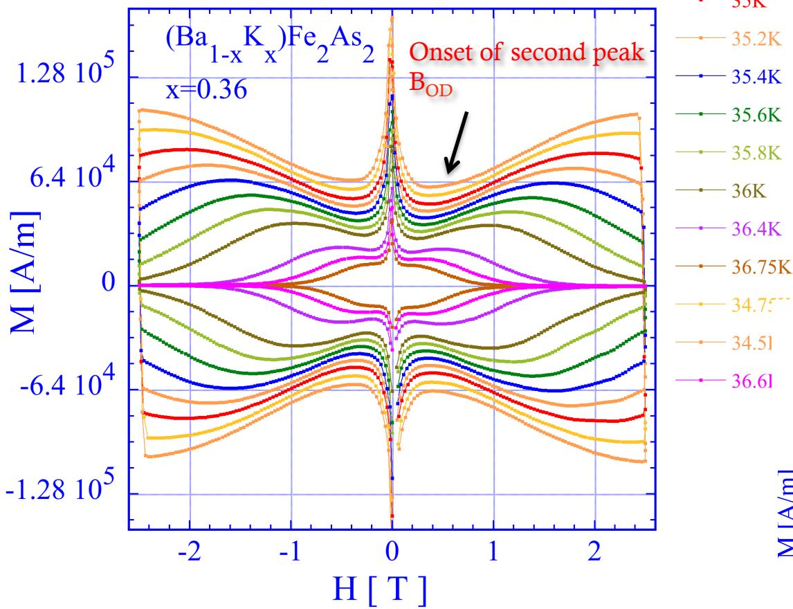
Different creep rates for different field phases can explain the M-H curves evolution in temperature !
