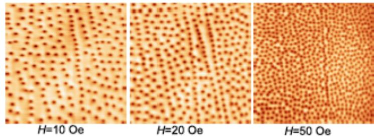
$\text{Ba}_{1-x}\text{K}_x\text{Fe}_2\text{As}_2$   $x=0.40$  MFM
